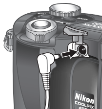
Connecting AC adapter to COOLPIX4500 DC-in connector
